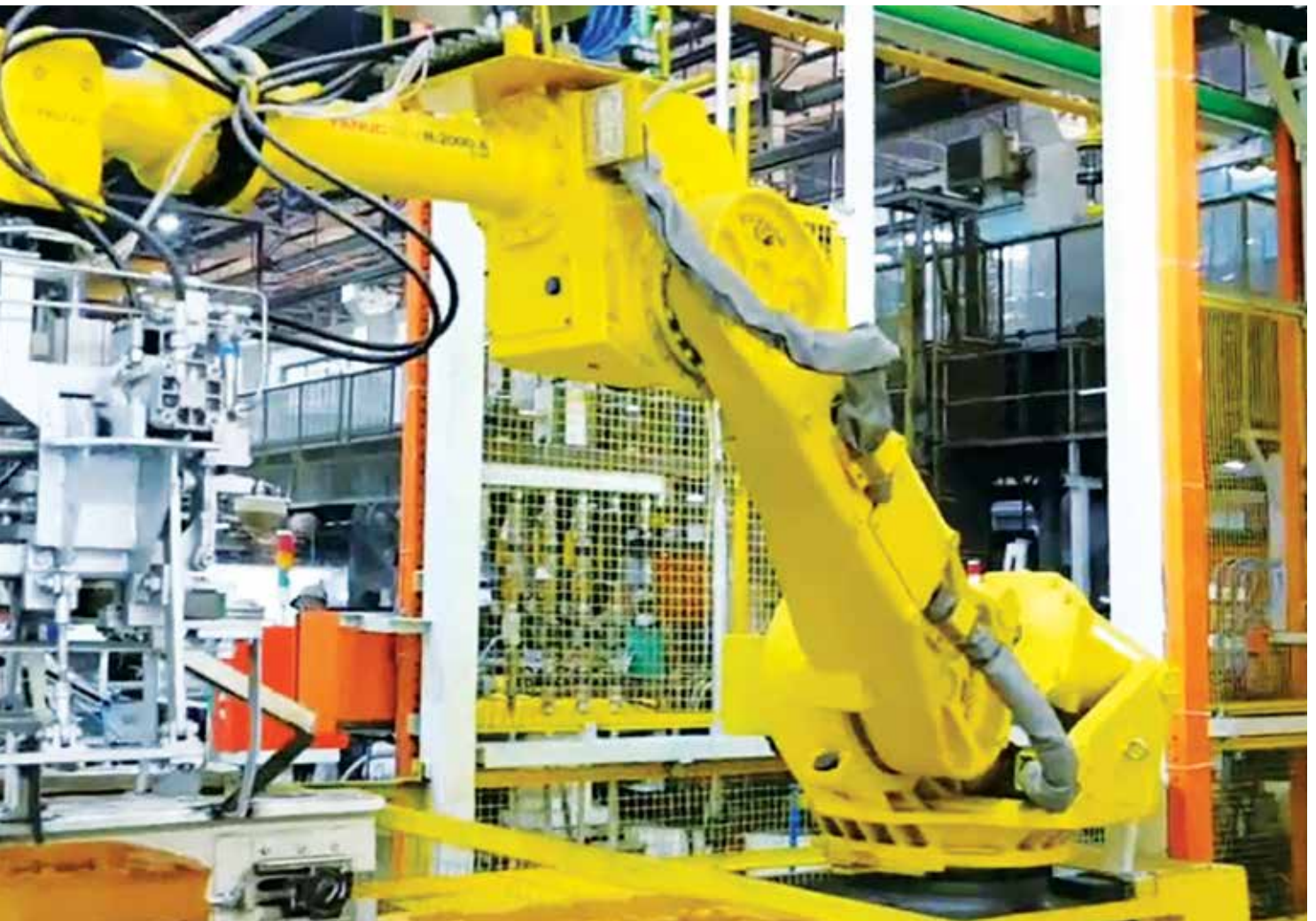
Automatic GDC production line with robots for 4W Cylinder head
