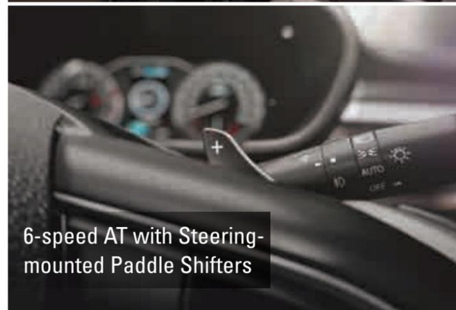
6-speed AT with Steering-mounted Paddle Shifters
