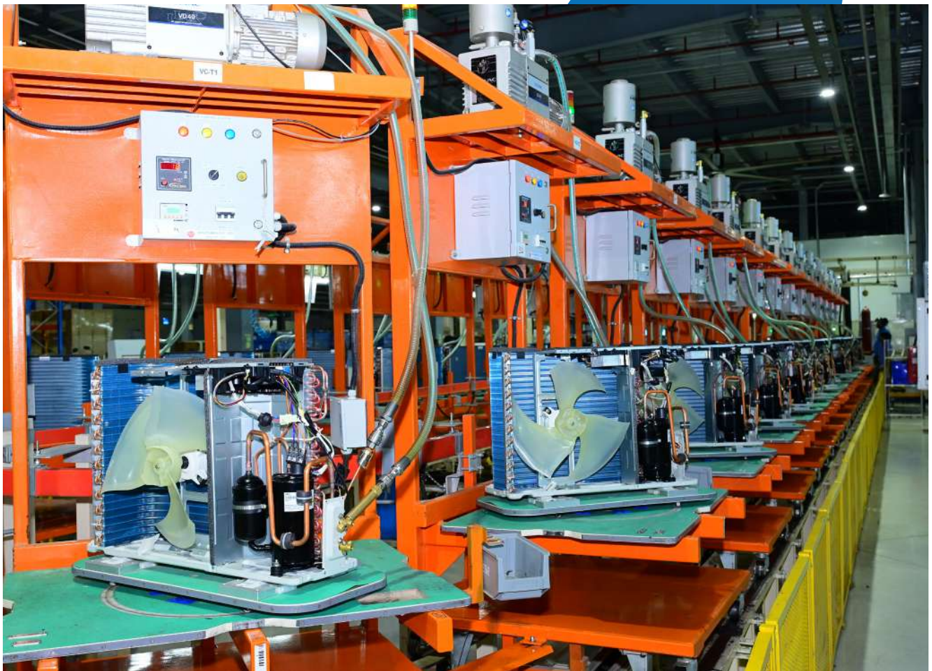
Outdoor Unit assembly conveyor belt at Sri City Plant
