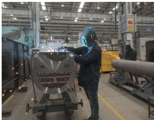
Precision welding of a chiller shell at Wada Plant
