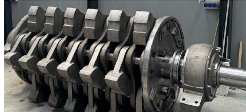
Hammer Crusher Rotor (54 MT)
