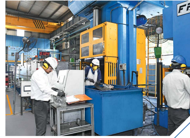
Manufacturing Axle Clamp and Underbracket Aluminium Forgings as a Backward Integration for Inverted Front Forks
