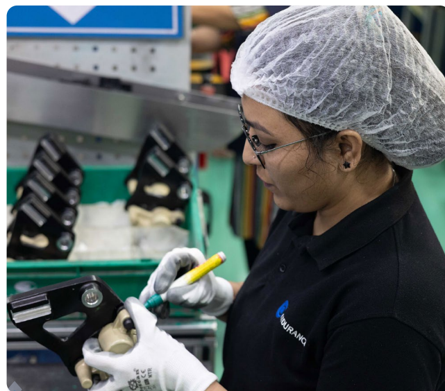
Final inspection of rear-caliper assembly at the disc-brake plant, Chh. Sambhajinagar.
