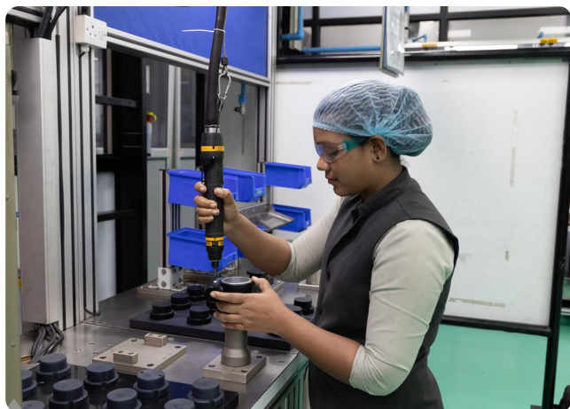
Torqueing operation at the suspension plant, Chh. Sambhajinagar
