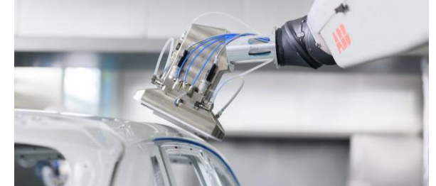
Robotics automation for painting and cleaning of EVs from a leading Indian auto major
