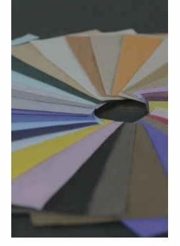
Spunbond fabrics are produced by depositing extruded, spun filaments onto a collecting belt in a random manner followed by bonding the fibers. The fibers are separated during the web laying process by air jets or electrostatic charges.
