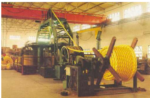
Production of 8-strand Mooring Rope
