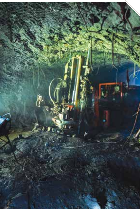
Longhole solo drill rig for accurate drilling
