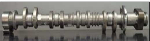
Hybrid Camshaft – Chilled Casting + Steel Fuel Lobe
