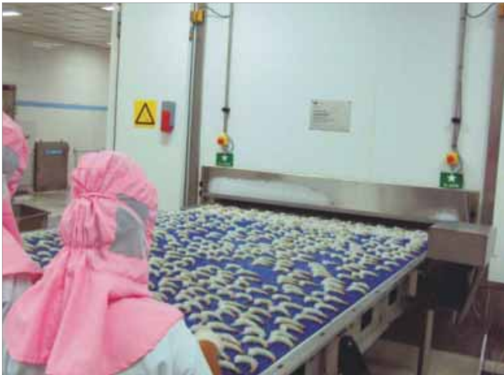
IQF machine in operation at Shrimp Processing & Export Plant located at Gopalapuram, East Godavari District, Andhra Pradesh
