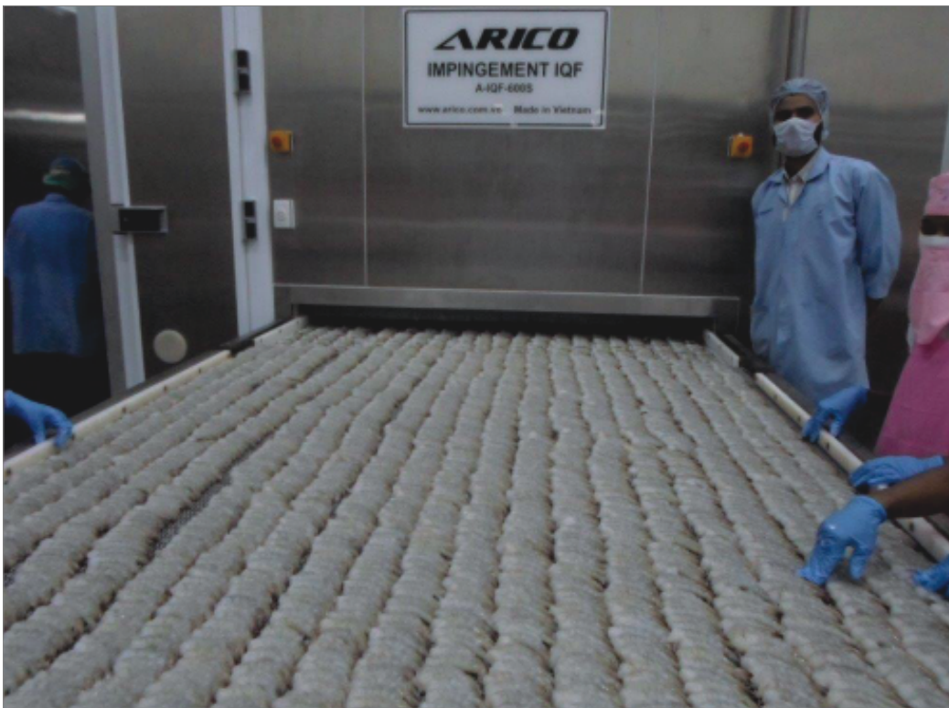
New IQF machine in operation at shrimp processing & export division at Gopalapuram.
