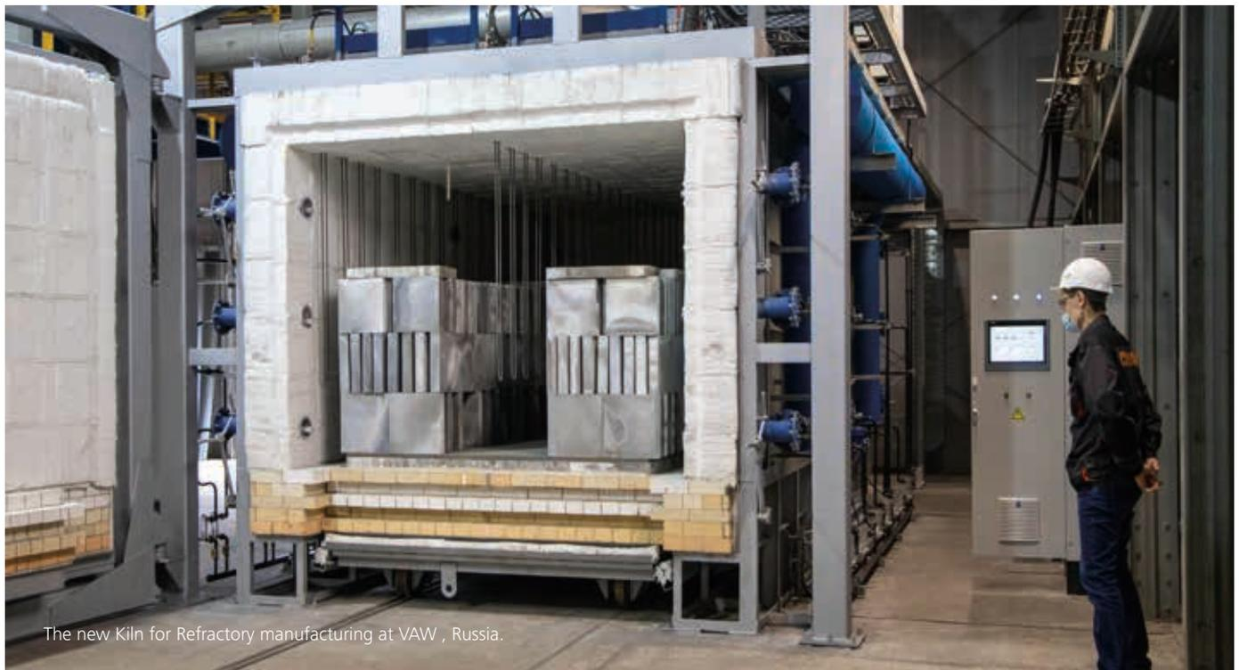
The new Kiln for Refractory manufacturing at VAW , Russia.
