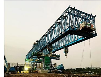
Launching Gantry (to lift and support bridge segments or girders) (S550MC – HR)
