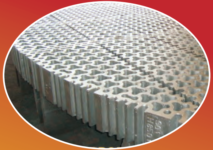
CHECKER SUPPORTING SYSTEM FOR HOT BLAST STOVES (BLAST FURNACE)
