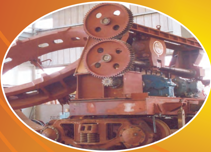
SLAG TRANSFER CAR FOR CARRYING HOT SLAG (BLAST FURNACE)
