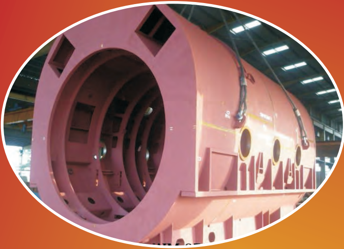
STATOR FRAME (270 MW GENERATOR)
