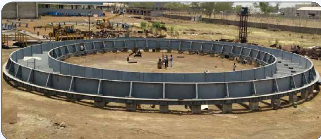
SINTER COOLER COMPLETE ASSEMBLY IS UNDER MANUFACTURING AT OUR FACILITY.
