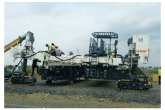
Writgen Slipform Paver used for pavement quality concrete
