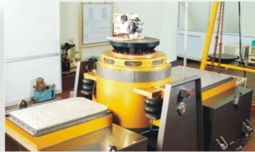
Vibration Resistance Testing
