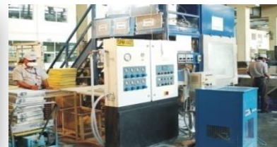
Nocloc brazing furnace for Condenser
