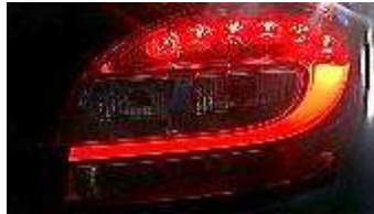
Tail Lamp with LED Signature and Tail function
