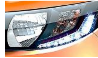
Head Lamp with bulb + Led DRL
