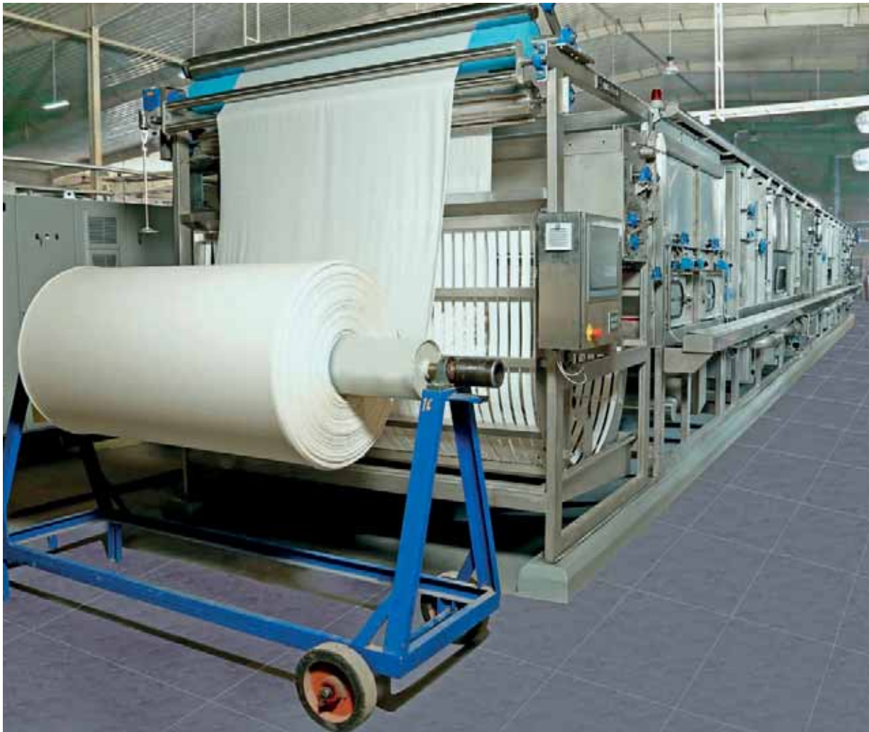
PLC based Washing Range
