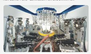
3 Layer Blown Film Co-ex Lines (upto 800 Kg/hr)
