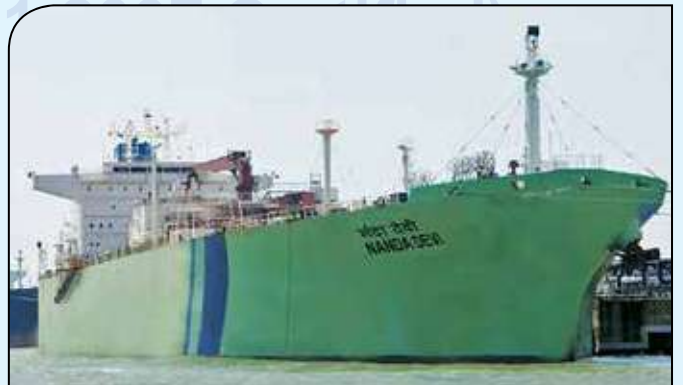
The Shipping corporation of India Ltd acquired second hand Very Large Gas Carrier (VLGC) 'Nanda Devi' on 14th September 2017 having a gross tonnage of 46,506 and deadweight of 53,503 tonnes
