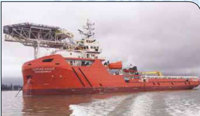
The Shipping corporation of India Ltd acquired second-hand Multi Purpose Support Vessel (MPSV) SCI Saraswati on 7 th July, 2017 having a gross tonnage of 3,616 and deadweight of 3719 tonnes
