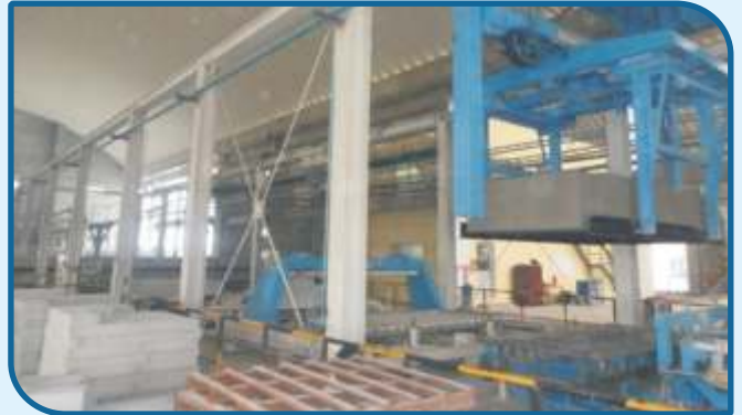
JK Lakshmi Cement SMARTBLOX (Autoclaved Aerated Concrete Blocks) manufacturing unit at Jhajjar
