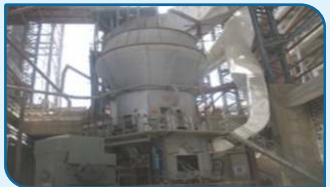
JK Lakshmi Cement initiative to optimise Chinese VRM at 210 TPH against rated capacity of 180 TPH
