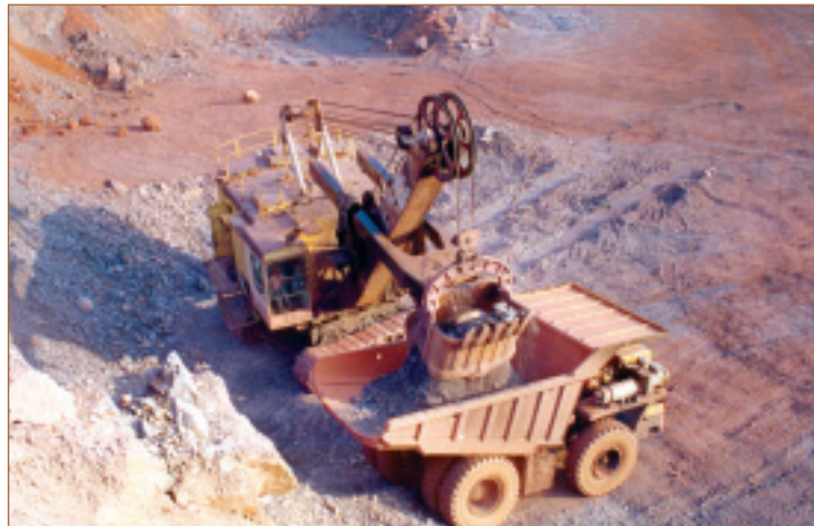
Shovel - Dumper operation
