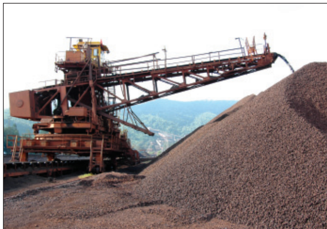
Stacker in Operation
