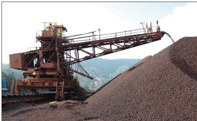
Stacking the CLO (Iron Ore) with Stacker at NMDC Loading Plant
