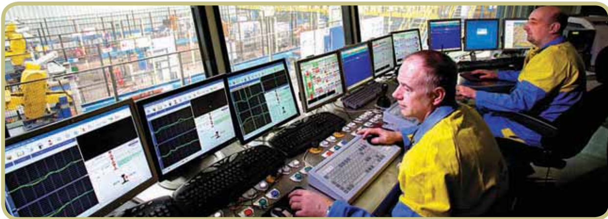
Saw pulpit at Scunthorpe Rail Service Centre
