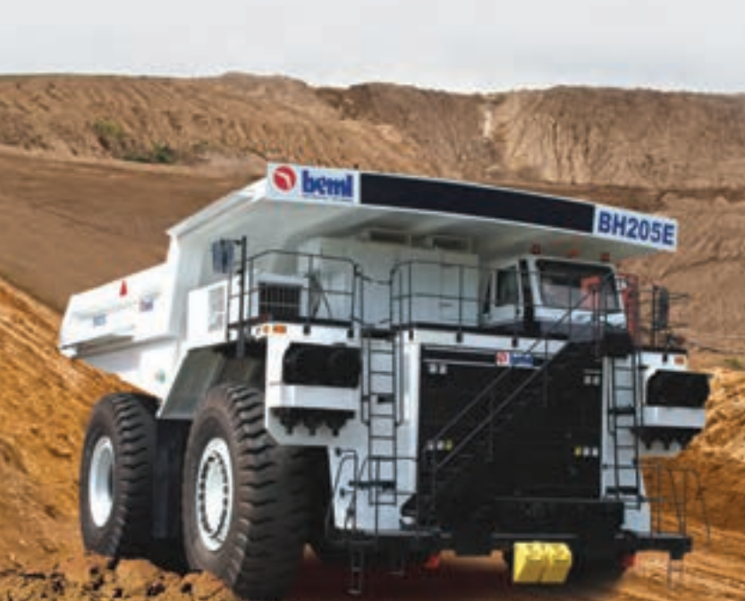
Reaching new heights - Inside India's largest Dump Truck is a Cummins engine: The largest dump-truck to ever be built in India by BHEL for Coal India, is being powered by a Cummins engine (60 litre). One of the highlights at the 'Make in India Week', this dump-truck was seen at close quarters by the Cummins Inc. COO and the India leadership (inset).
