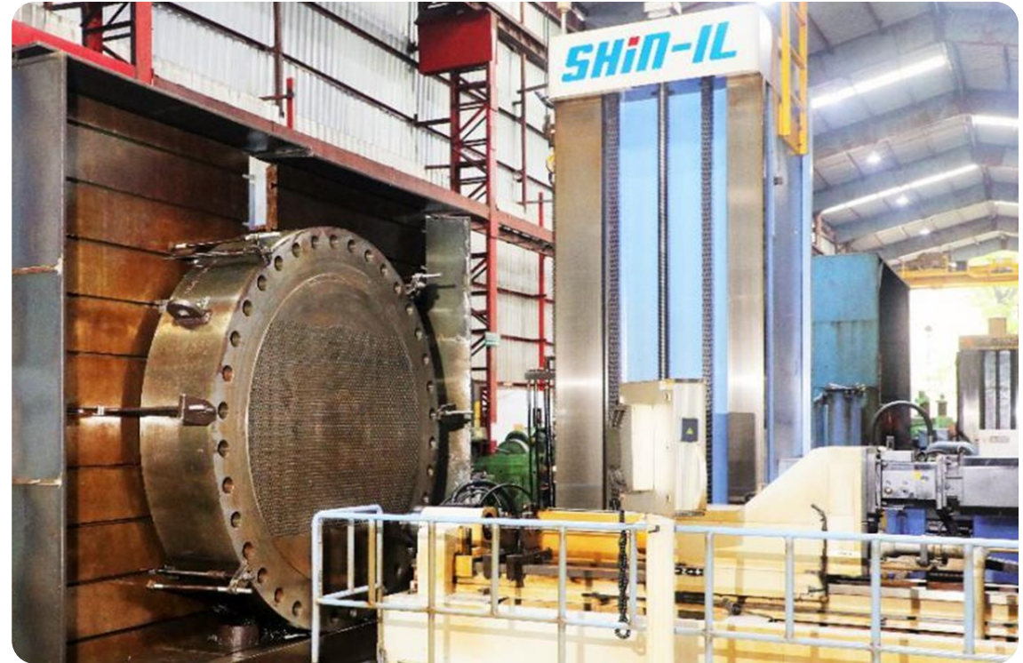
1500 mm thk CNC Deep Hole Drilling
