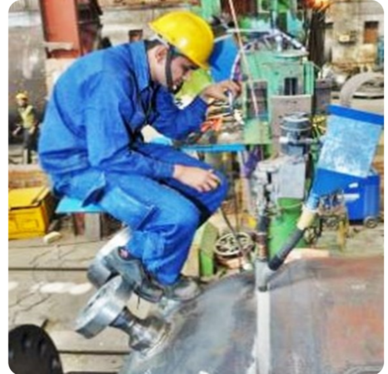
Narrow Gap Welding (J-Groove)
