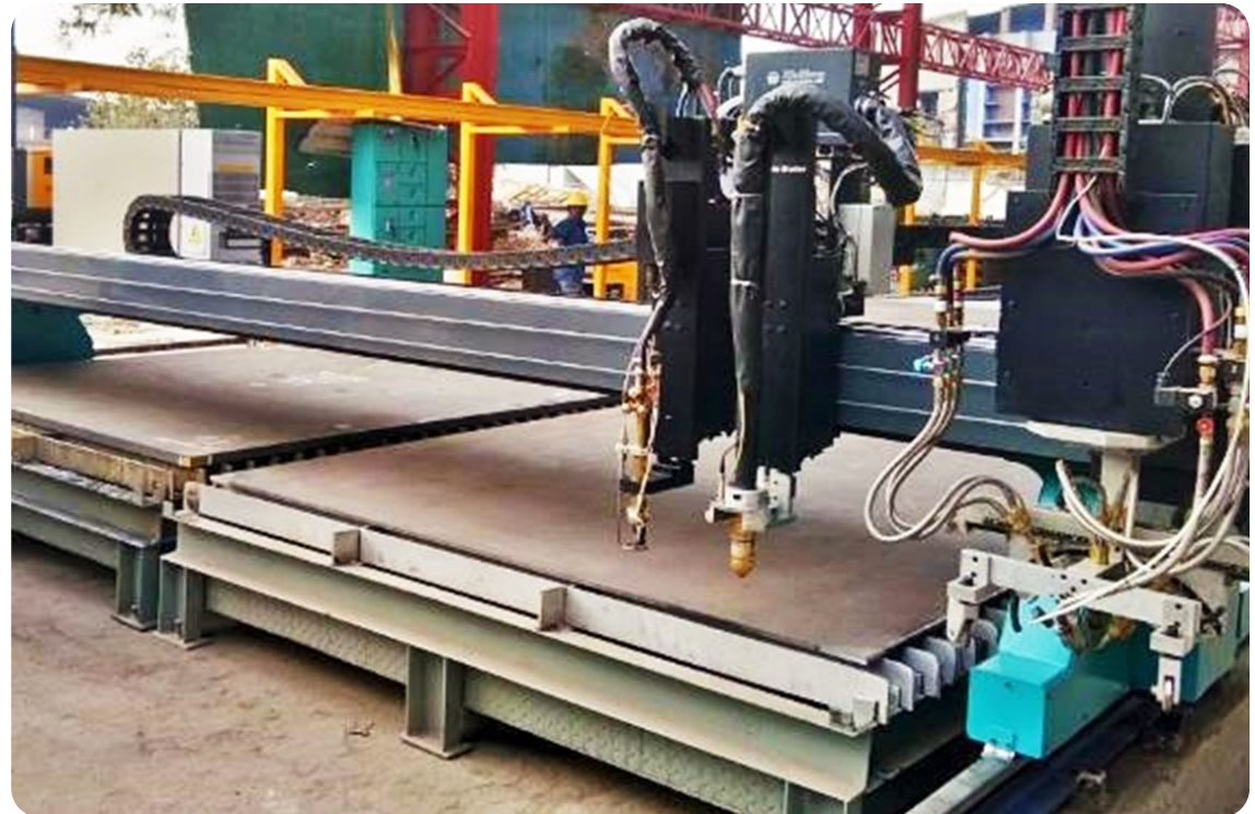
CNC Plasma Cutting – upto 300 mm CS
