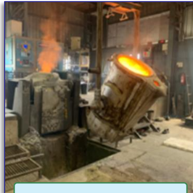
Induction Furnace 550 KW, 500 KG
