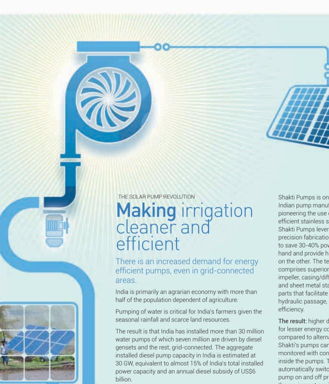
Shakti Pumps is one of the largest Indian pump manufacturers, pioneering the use of energy efficient stainless steel pumps. Shakti Pumps leverages advanced precision fabrication technology to save 30-40% power on the one hand and provide higher output on the other. The technology comprises superior hydraulic impeller, casing/diffuser designs and sheet metal stainless steel parts that facilitate smooth hydraulic passage, ensuring high
