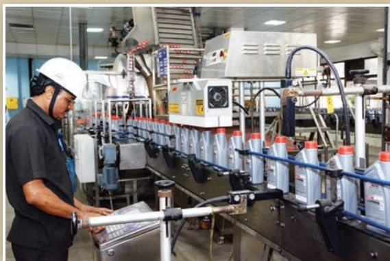
The high speed small pack filling line
