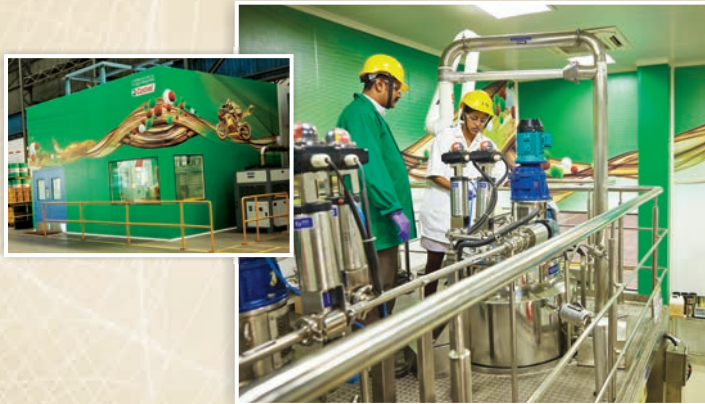
Castrol has set up a pilot blender at its Silvassa Plant to enable new product development, specially for OEM partners
