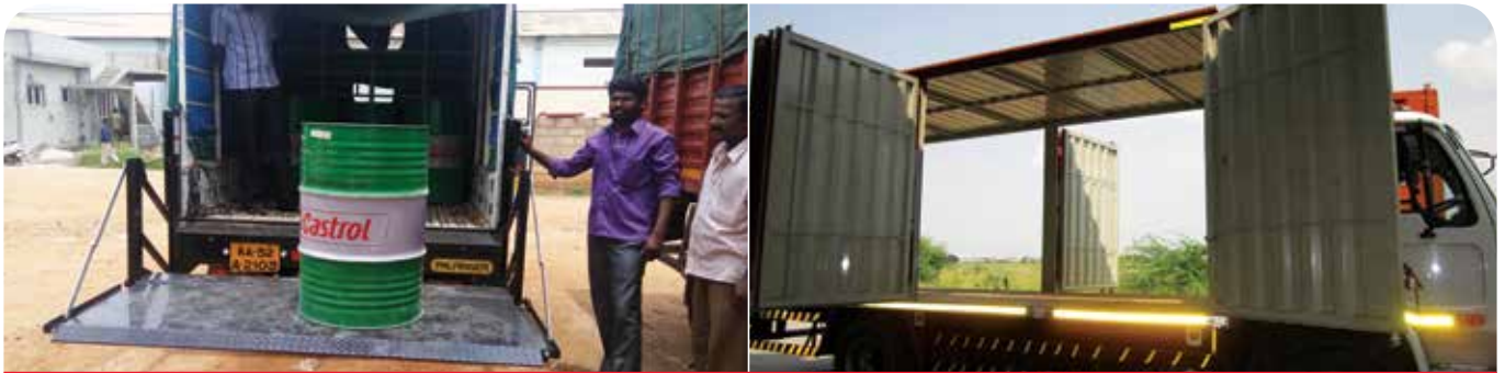
In its continuous endeavour to extend safety beyond its own sites, Castrol launched two innovations for the first time in India. Photograph on left shows a hydraulic tail lift developed to ensure safe handling of barrels. Photograph on right shows a three side open vehicle specially designed for a key OEM to enable safe and efficient handling of products
