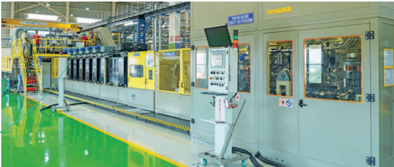
First in the world - Stamped grid manufacturing line commissioned in the newly built motorcycle battery plant
