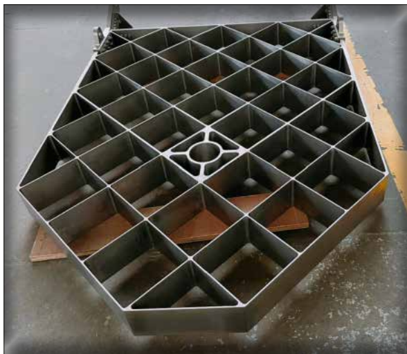
Grid Fin Structures for Gaganyaan, India's first human flight mission
