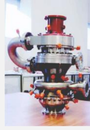
Cryogenic Engine - Turbo Pump, Injector Head, Gas Generator, Booster Pumps, Interfaces And Start Up Systems
