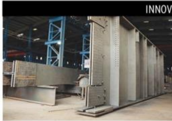
Fabricated Structures Sections: H-type Beam, I-type Beams, Box Sections and Star Couiums Sections: Depth: 350mm - 3000mm, Flange Width: 250mm - 1000mm, Length: 3 to 18 meters
