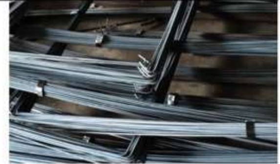
Cut & Bend Customized and Ready to Use TMT Rebars
