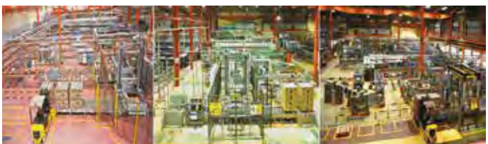
Bottling Line 2: 36000 bottles per hour
