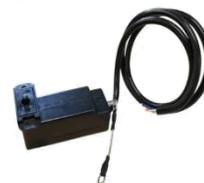
Charger Lid, Seat Latch, Steering Lock Actuators
