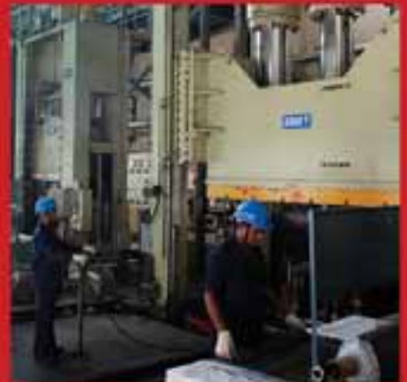
2000 T MOULDING PRESS AT COMPOSITES, PUNE
