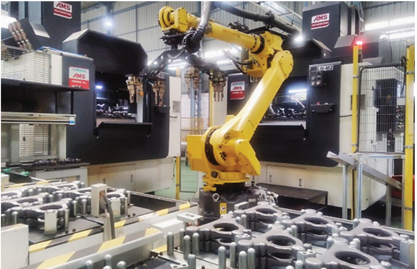
▲ Heavy Duty Flange Automated line at Bill Forge, Bengaluru
