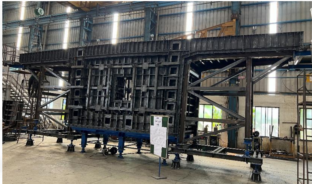
Pier Head Segment
