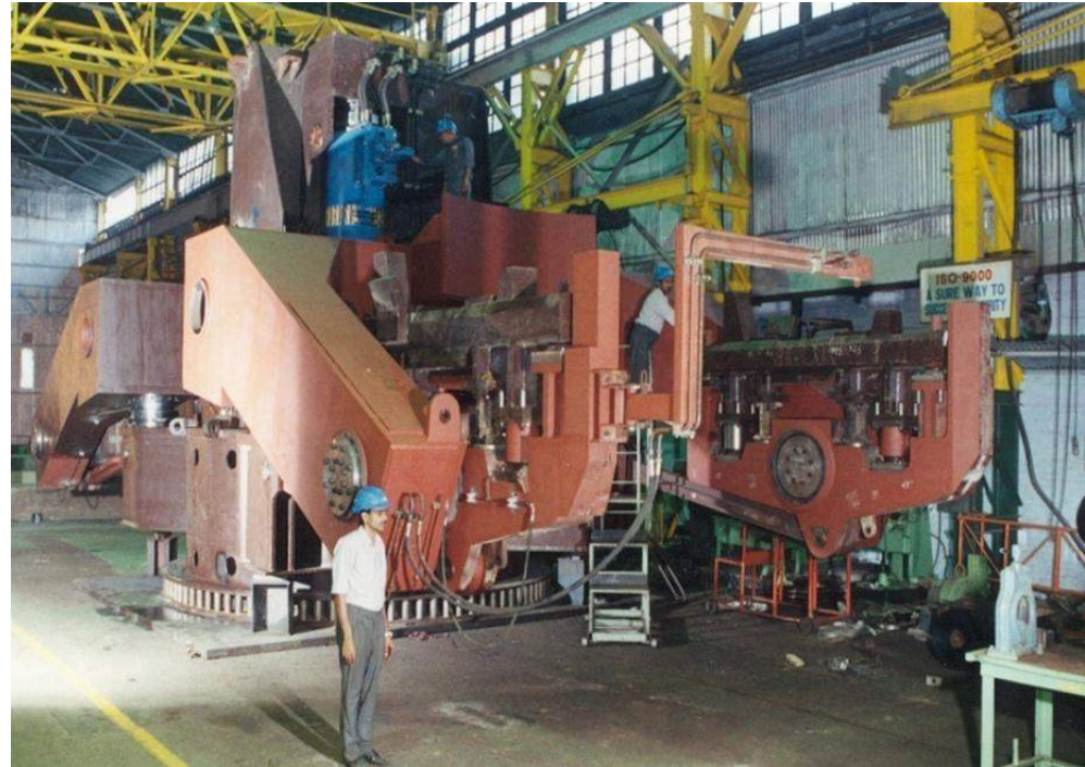
Ladle Turret for 2 ladles - 165 T each Design : SMS Demag
