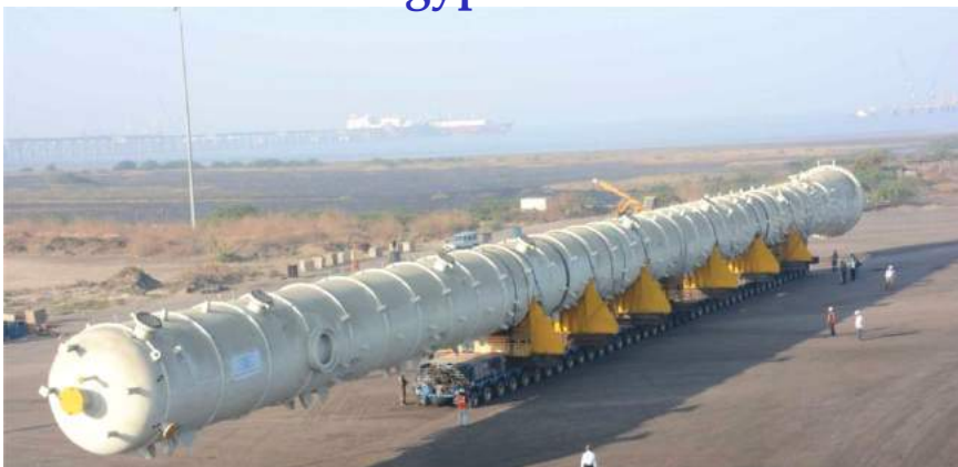
105 M Long Ethylene Fractionator for Customer in Egypt
