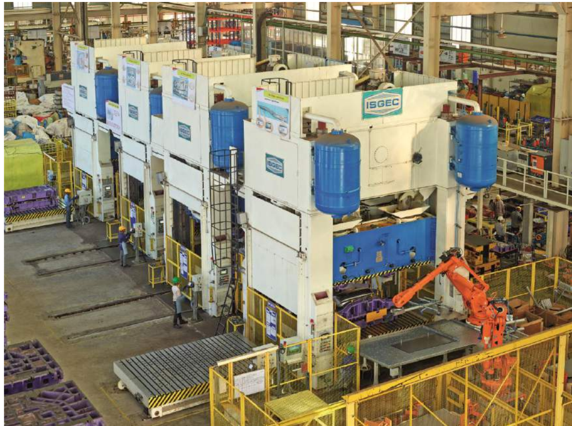
1000 T Robotic Tandem Press Line supplied to Auto Company in Telangana, India
