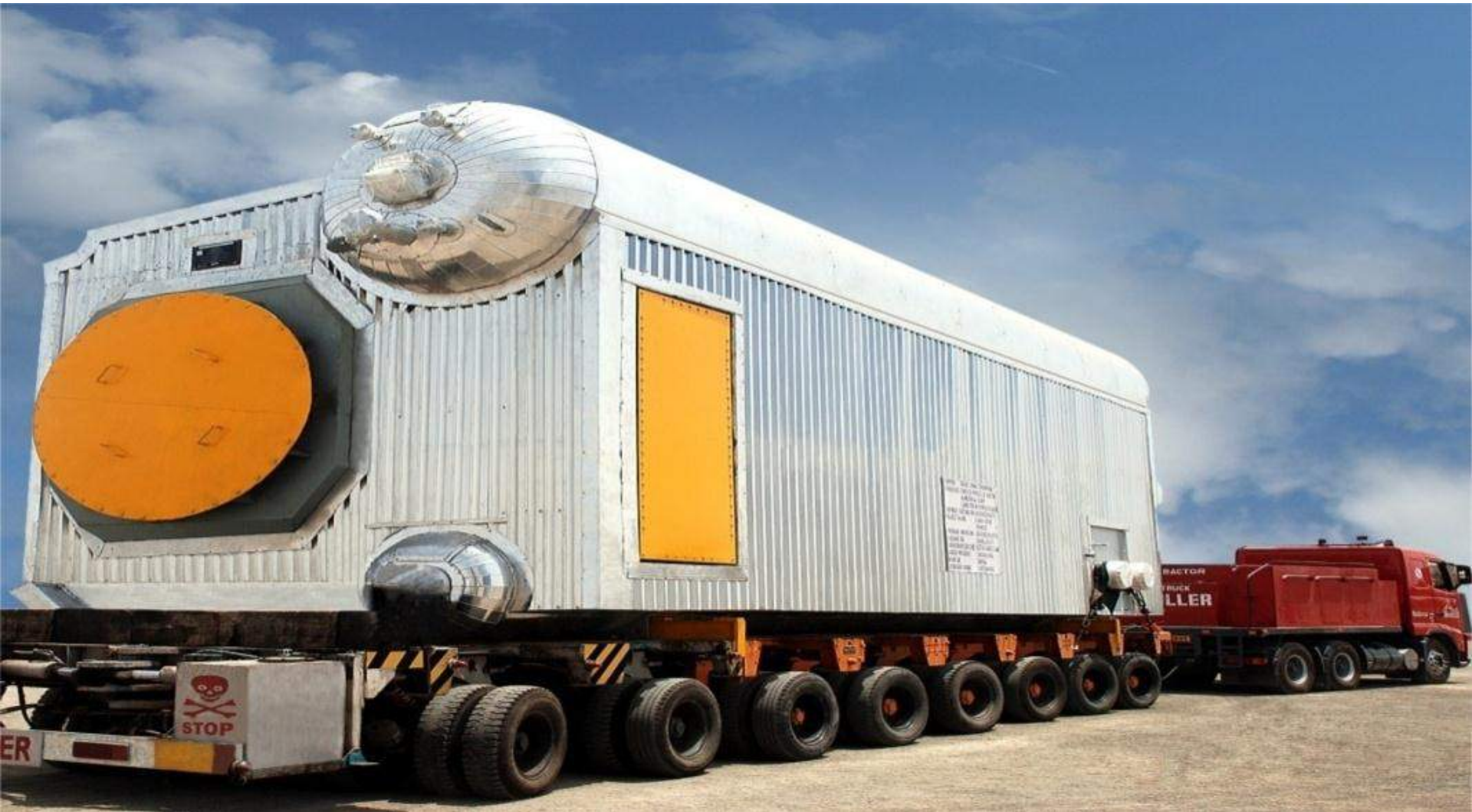
77 TPH Package Type Oil & Gas Fired Boiler
