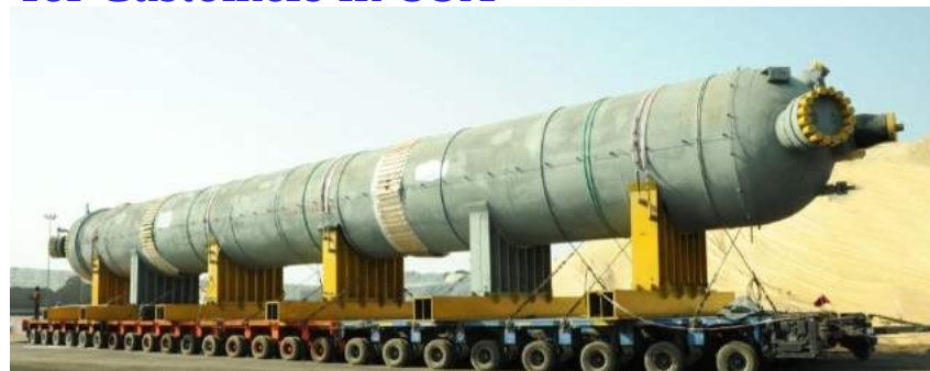
817 MT, Ammonia Converter, with Internals for Customers in USA
