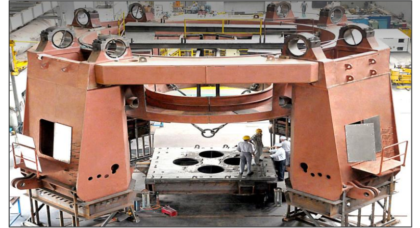
Mill stands, as per design of Loesche, Germany
