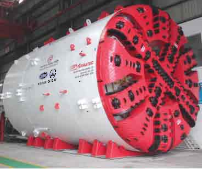
Tunnel Boring Machine
