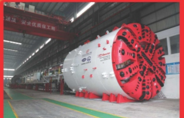
Tunnel Boring Machine
