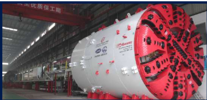
Tunnel Boring Machine (TBM)
